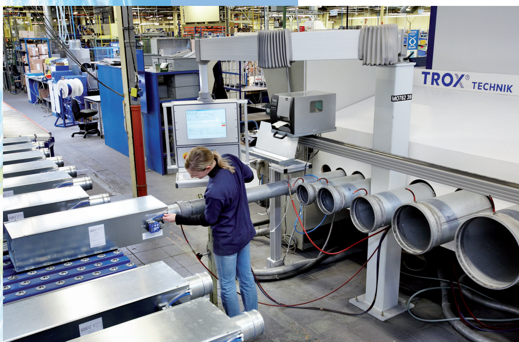
Manufacturing and adjusting air terminal units
