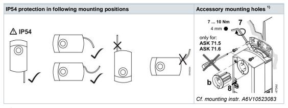
$oldsymbol{\Lambda}$   $^{1)}$ Not to be used for fixation of the actuator, use anti-rotation-bracket instead.
