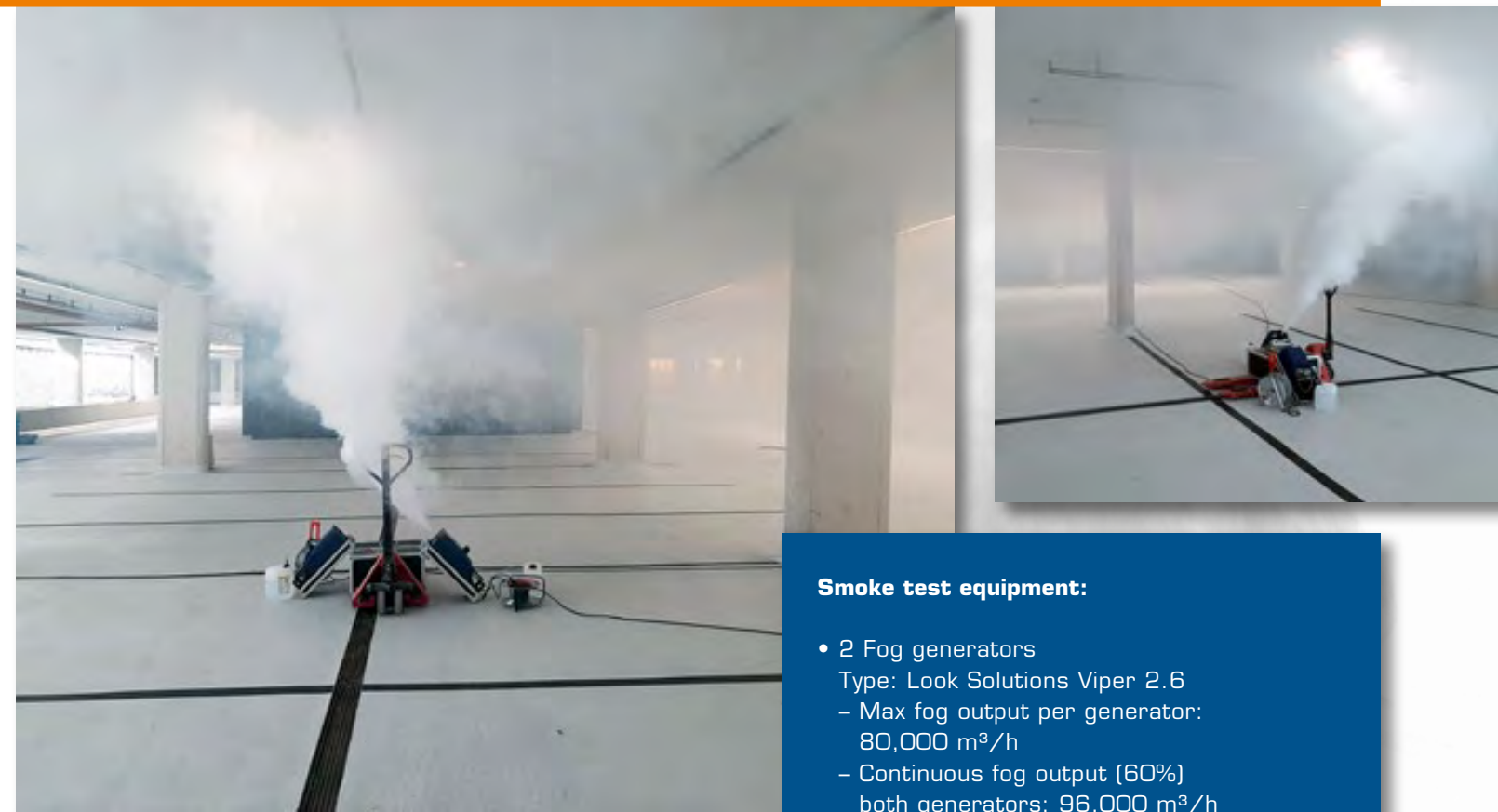
Smoke tests using fog generators and, in some cases, gas heaters to increase the temperature.
